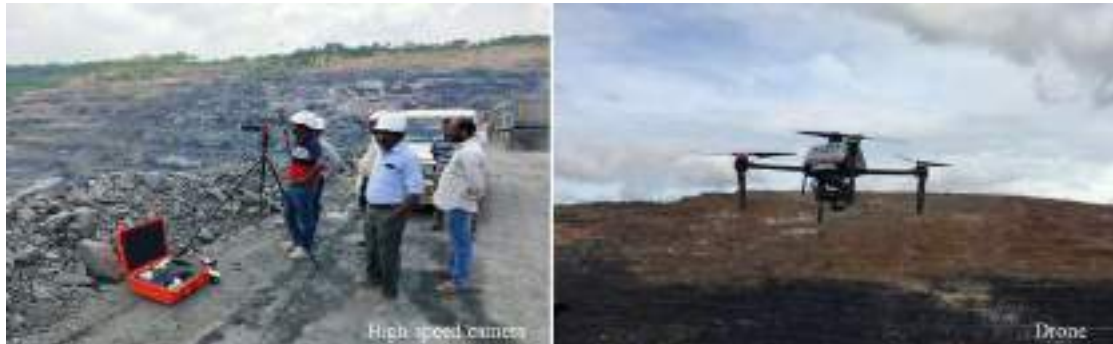
High speed camera and drone were used to optimize the blast design
