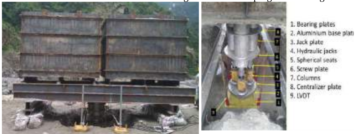
Plate load test setup for determining safe bearing capacity
