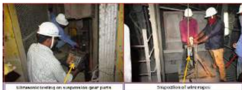
NDT on winder suspension gear parts and wire ropes, M/s HCL.
