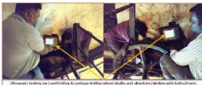
NDT on EOT crane vital components, M/s KPCL, Shivanasamudram
