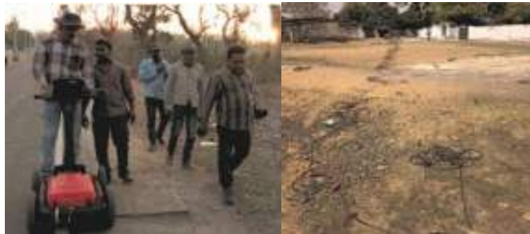
Geophysical survey in progress using GPR (left) and MASW techniques (right)
