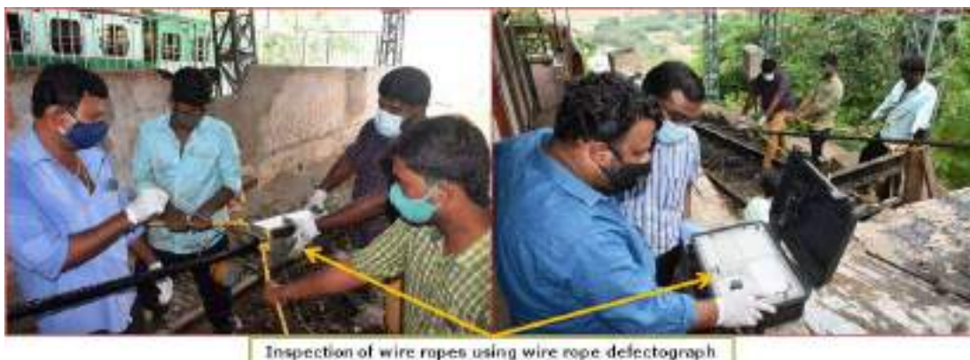
Inspection of winch ropes using wire rope defectograph
