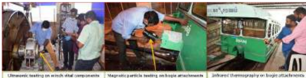
Testing of winch vital parts and bogie attachments
