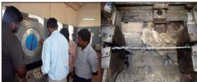
Testing of 14mm, RHL rope witnessed by representatives of M/s IMS & Ashok Leyland at NIRM laboratory
