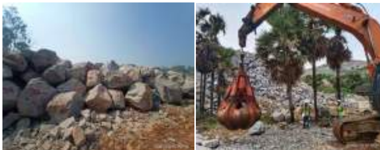
View of stock pile (left), Drop test for 1 ton armour rock (right)
