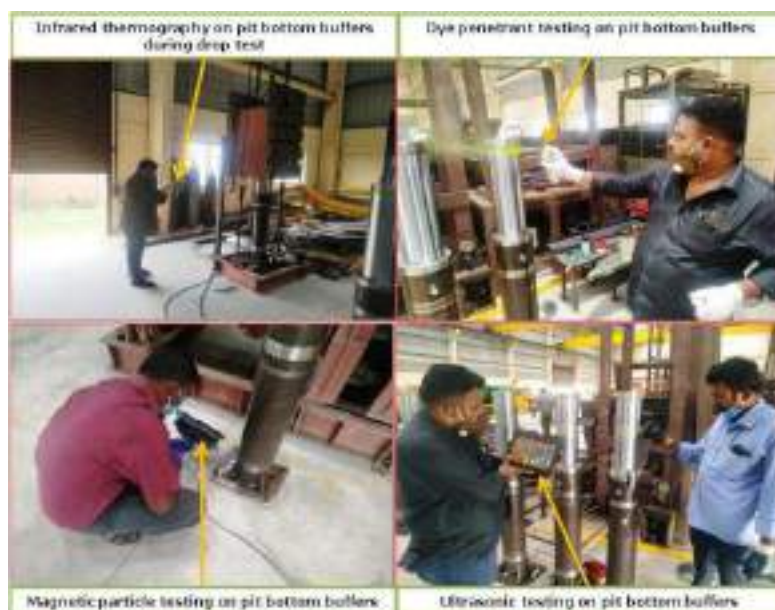
Testing of pit bottom buffers
