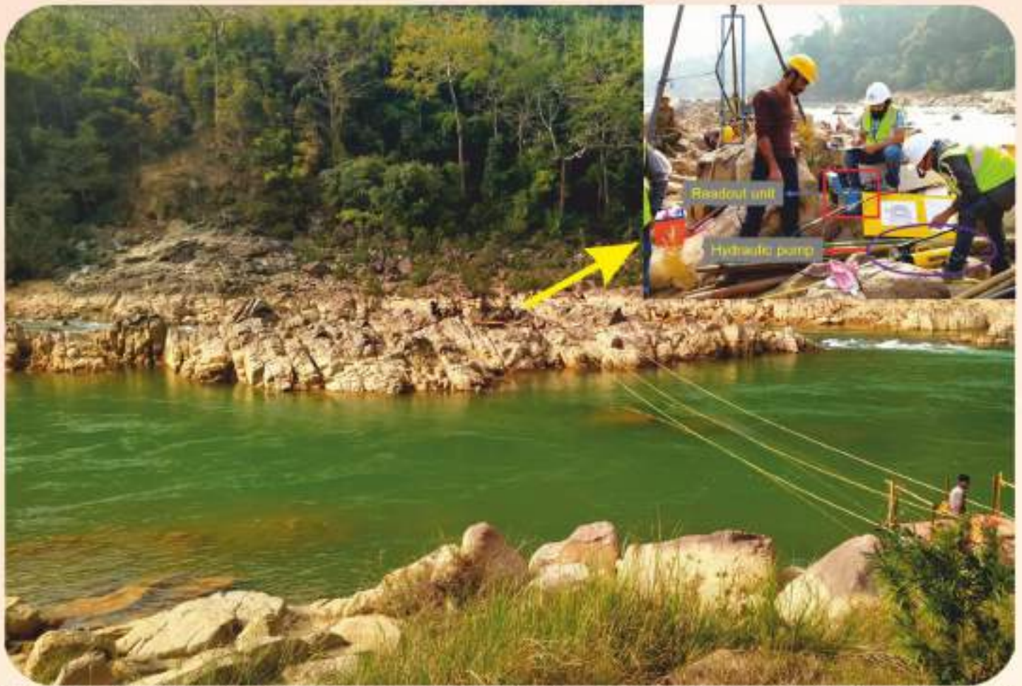
Goodman jack test conducted in a bore hole drilled at the centre of the river bed of lower Kopili hydroelectric project Assam. Inset showing the closeup view during test.
