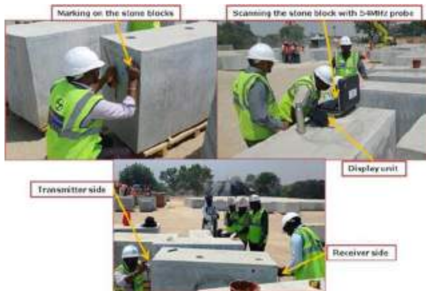
Some of the techniques used for quality assessment of stone blocks
