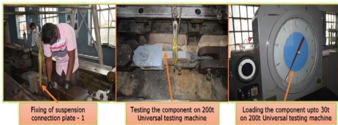
Testing of suspension connecting plate
