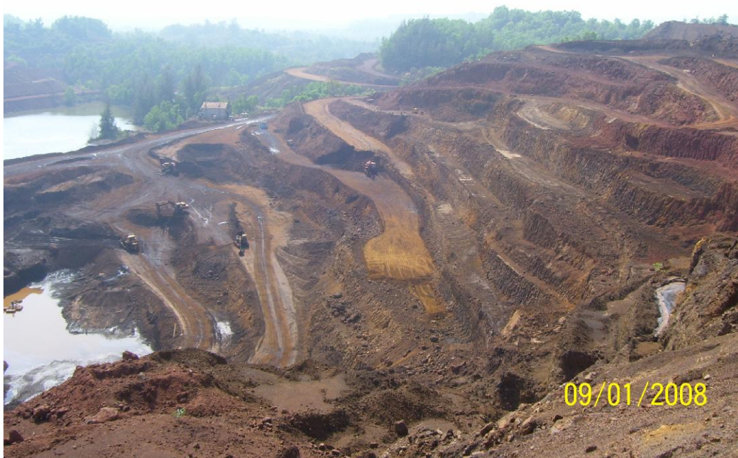
Fig. 8.6 Laterite at the top and soft clay below it, forming weak benches at an iron ore mine in Goa
