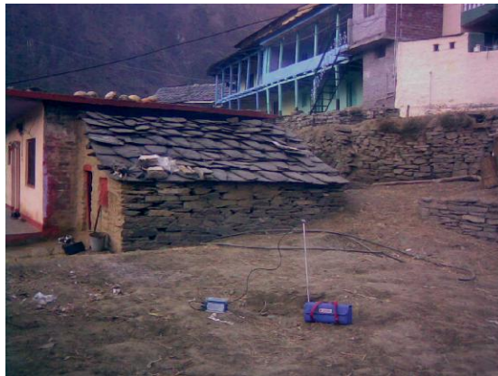
Fig. 7.6 Blast monitoring near a house at Brail village
