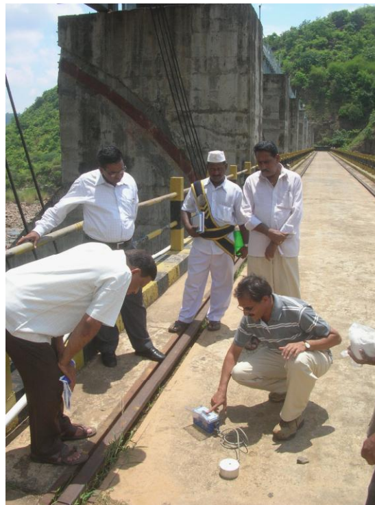
Fig. 7.2 Monitoring of ground vibration and air overpressure at Yeleru dam, A.P.
