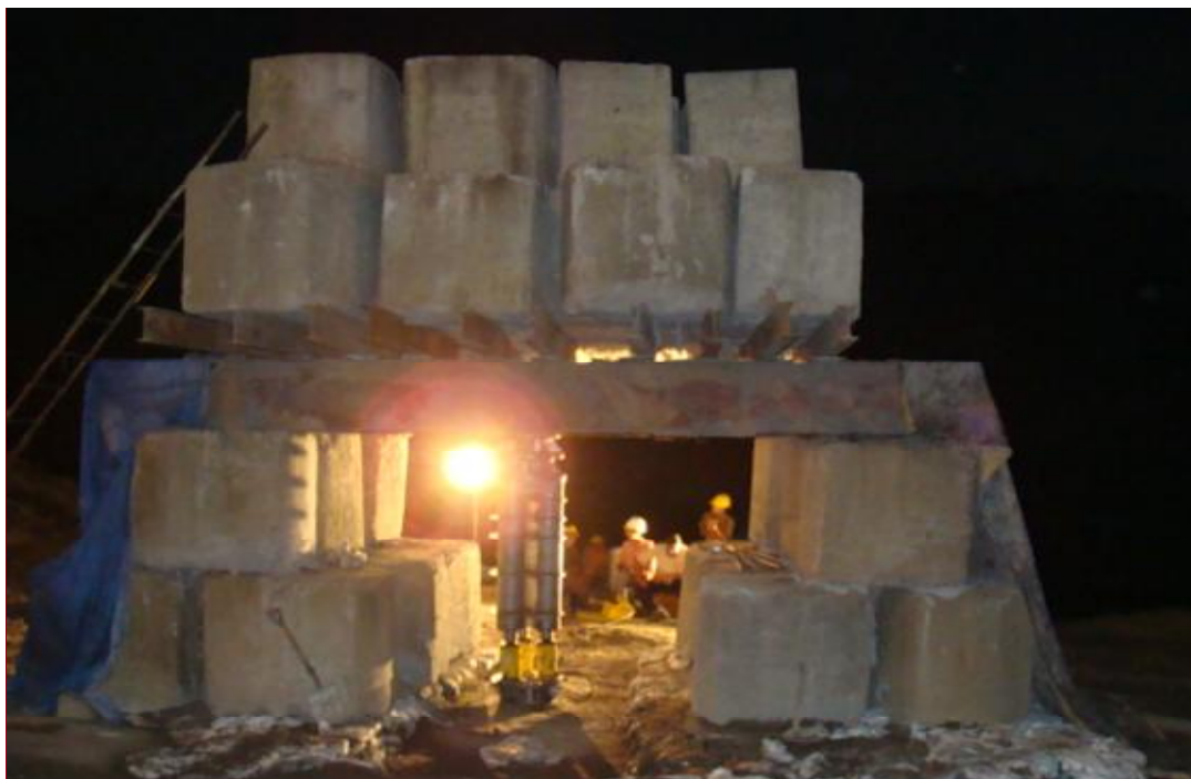
Fig. 3.4 Plate load experimental set-up at Subansiri Lower H.E. Project site
