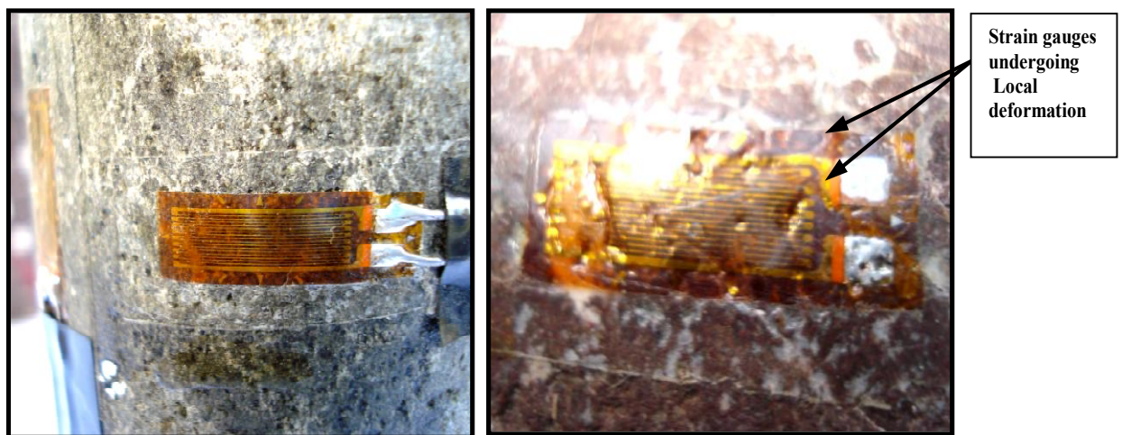
Fig. 4.2 Measurement of strain under triaxial conditions
