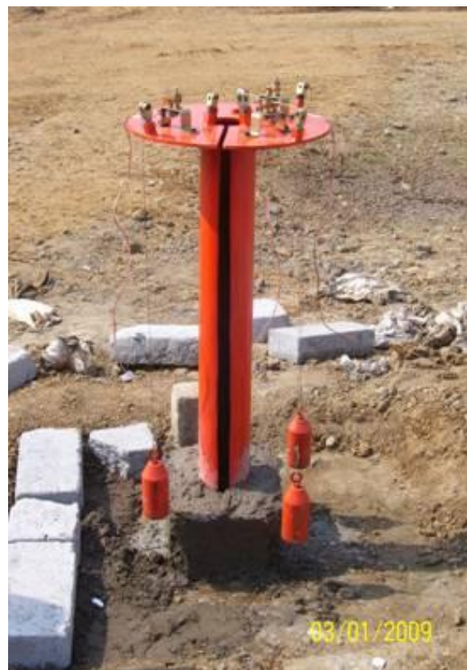
Fig. 8.4 Deep hole extensometers installed above the longwall panel
