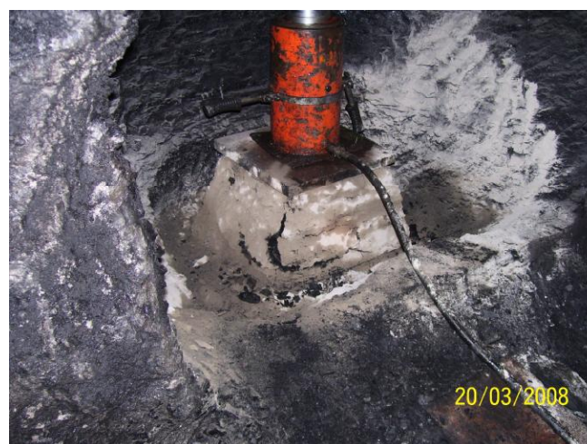
Fig. 8.2 Test set-up for determining in-situ strength of coal
