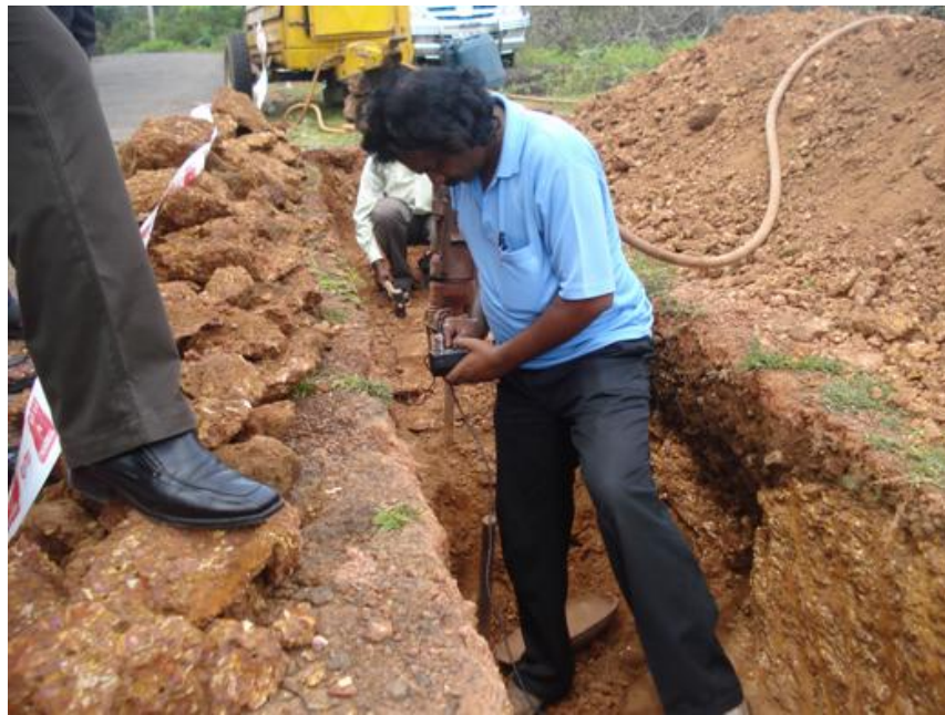
Fig. 9.1 P-wave velocity measurements in the trench
