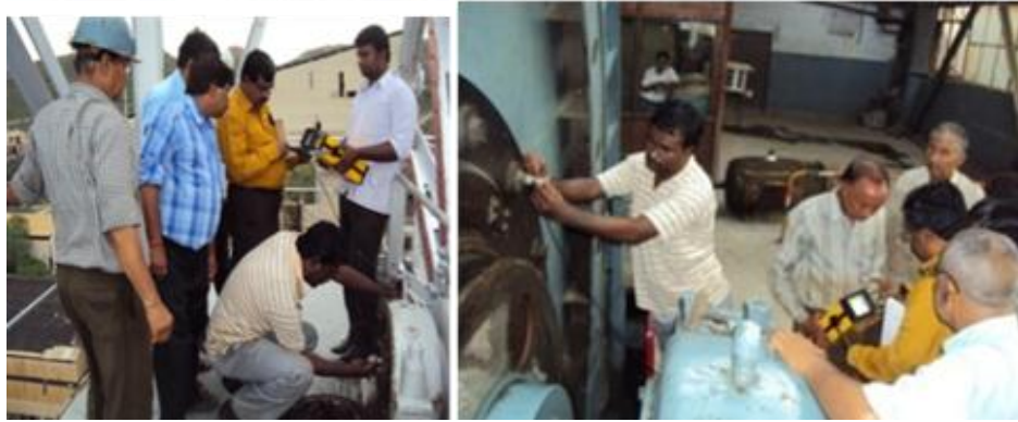
Fig. 12.7 NDT on winder vital components
