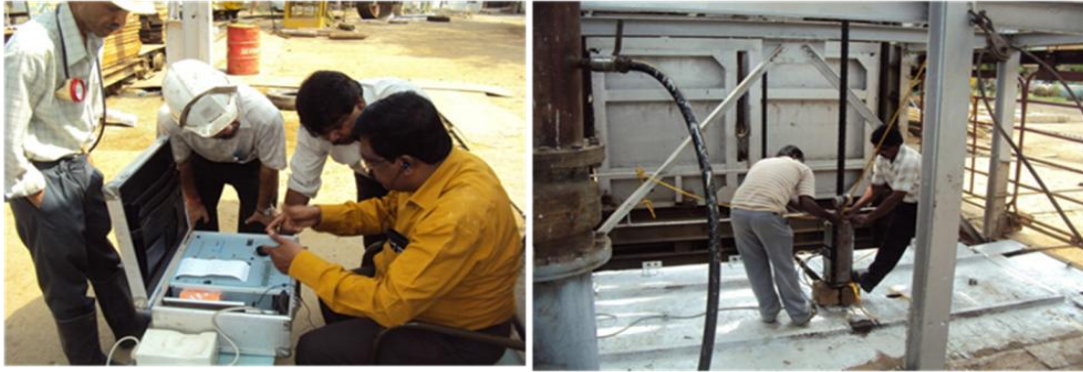
Fig. 12.8 Testing of rope using Defectograph
