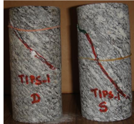
Fig. 4.2 Foliation planes with respect to core axis
