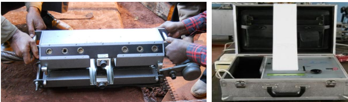
Fig. 12.5 Wire rope tester head unit and recorder (defectograph)
