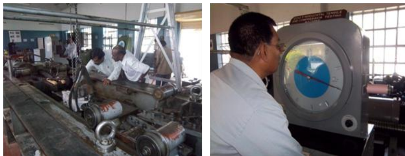
Fig. 12.1 Proof load testing of bracket assembly for white metal rope cappel
