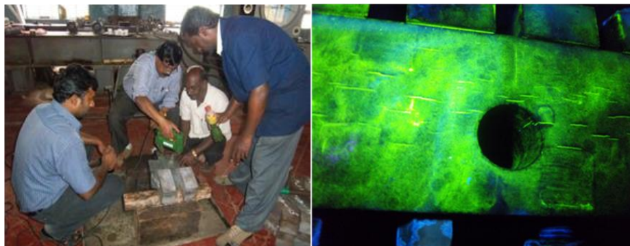
Fig. 12.2 Magnetic particle testing
