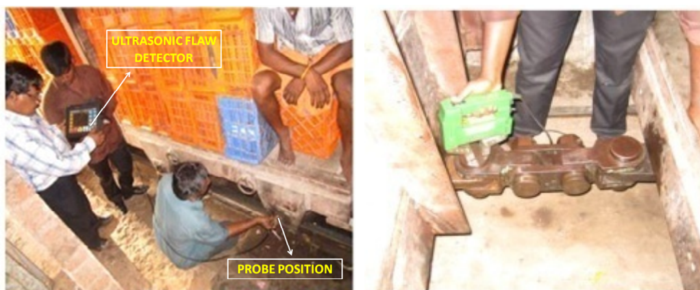
Fig. 9.3 NDT of winch and vital components at M/s Palani Temple, Tamil Nadu
