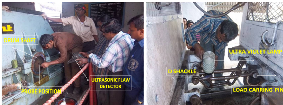
Fig. 9.1 NDT of winder vital components at M/s SCCL
