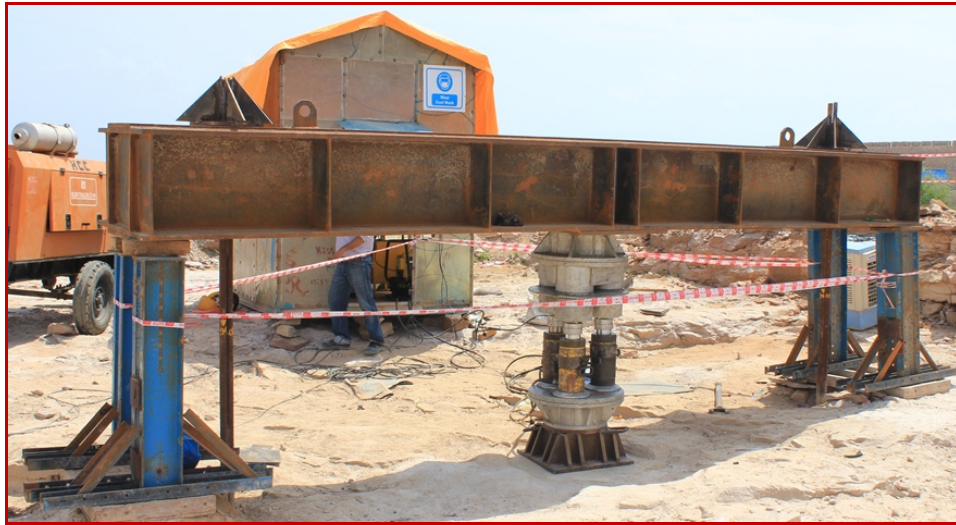
Fig. 3.1 Typical set-up for in-situ deformability investigations
