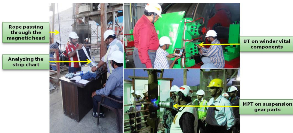
Fig. 9.6 NDT on winder vital components, suspension gear parts and wire rope inspection
