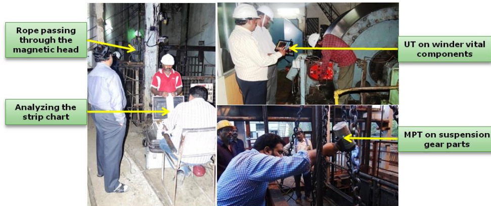
Fig. 9.3 NDT on winder vital components, suspension gear parts and wire rope inspection
