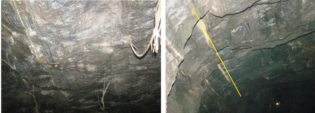
Fig. 7.2 Banded texture (foliation) in ore zone, and lineation and bedding planes at Chikla mine, MOIL Ltd
