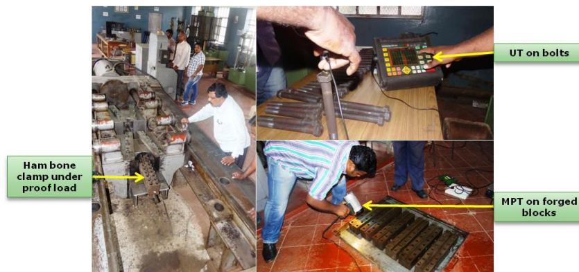
Fig. 9.7 Proof load test and NDT on 16 bolt ham bone clamps
