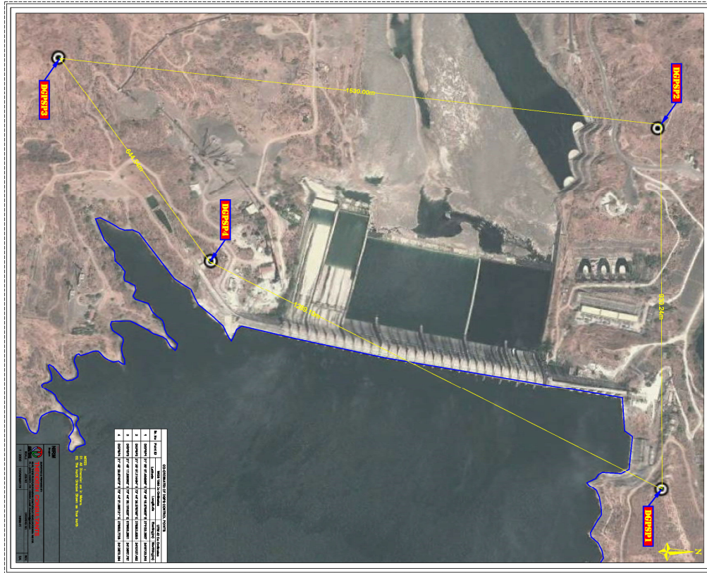
Fig 5.1 Control points network at SSNNL Dam
