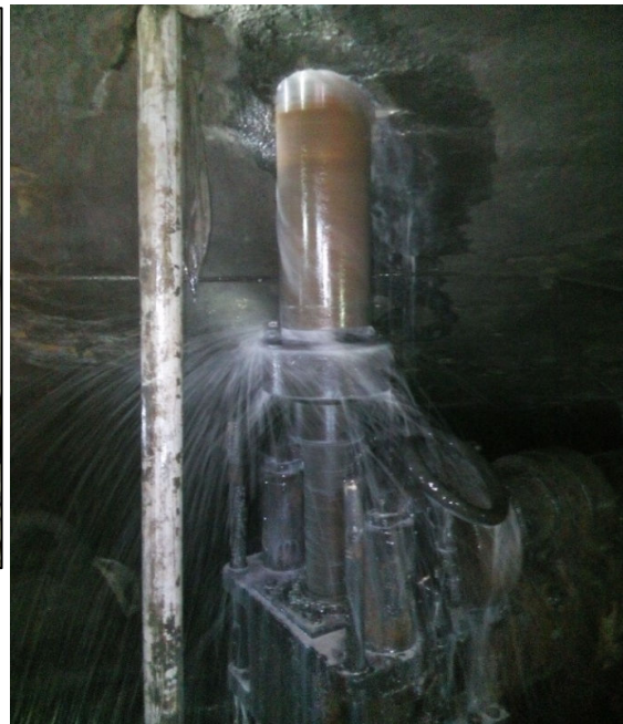
Fig. 3.5 Overcoring test at KTK-8 Incline
