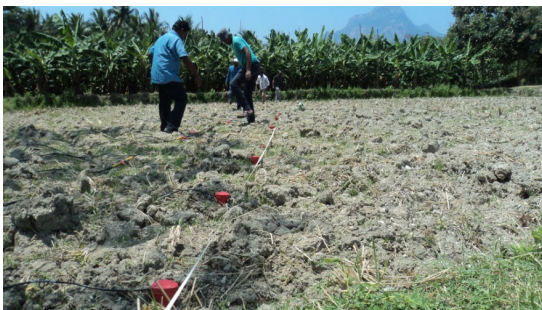
Fig. 4.1 MASW survey carried out across L2 lineament
