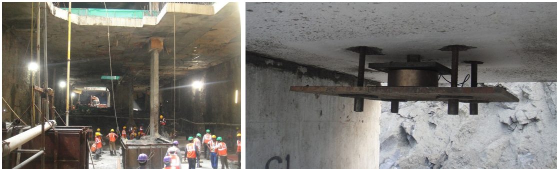
Fig. 6.9 Photograph showing blasting to be carried out under an RCC roof Fig. 6.10 Load cell mounted inside roof of the precast concrete structure at an alternate site to monitor load exerted by the explosive pressure
