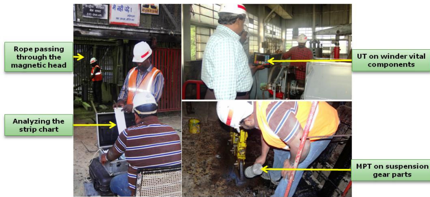
Fig. 9.8 NDT on winder vital components, suspension gear parts and wire rope inspection
