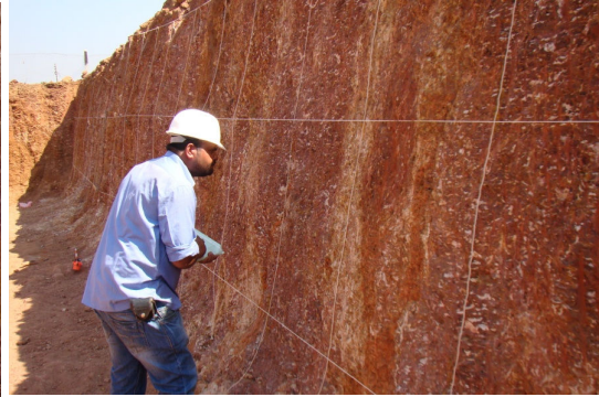
Fig. 4.7 View of 1 m X 1 m grid for mapping fine geological details
