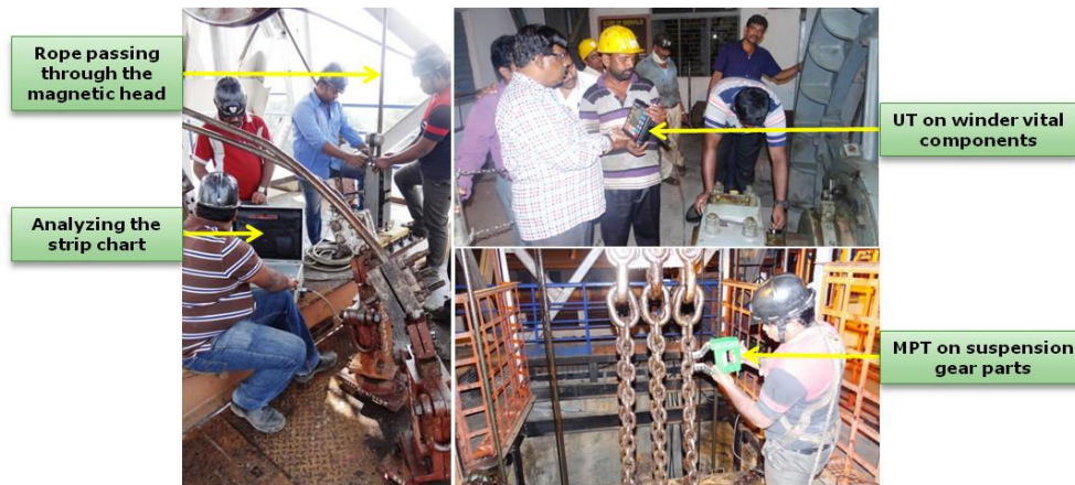
Fig. 9.5 NDT on winder vital components, suspension gear parts and wire rope inspection of various mines
