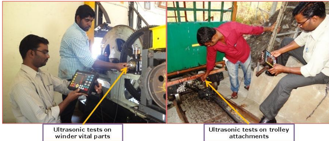
Fig. 8.17 NDT on winder vital components & trolley attachments, M/s KPCL
