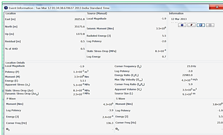
Fig. 7.2 Computed source parameters of a recorded microseismic event
