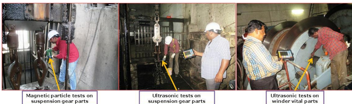
Fig. 8.11 NDT on winder vital components & suspension gear parts, Rajpura Dariba Mines, M/s HZL
