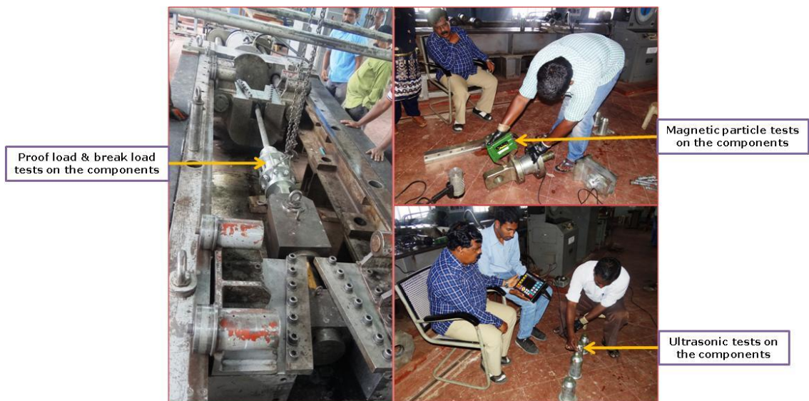
Fig. 8.16 Proof load test, NDT & break load tests on the suspension devices, M/s NFC
