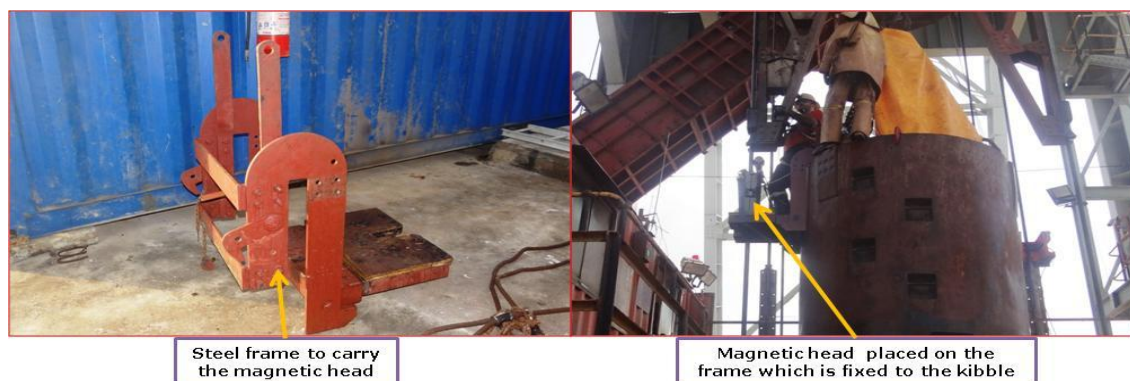
Fig. 8.3 Testing of stage winder ropes, M/s SSM
