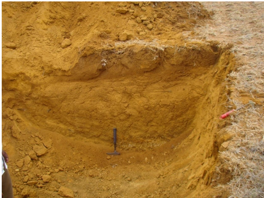
Fig. 1.14 Very soft sediment exposed in the velocity zone 400 m/s at Udaiyattur
