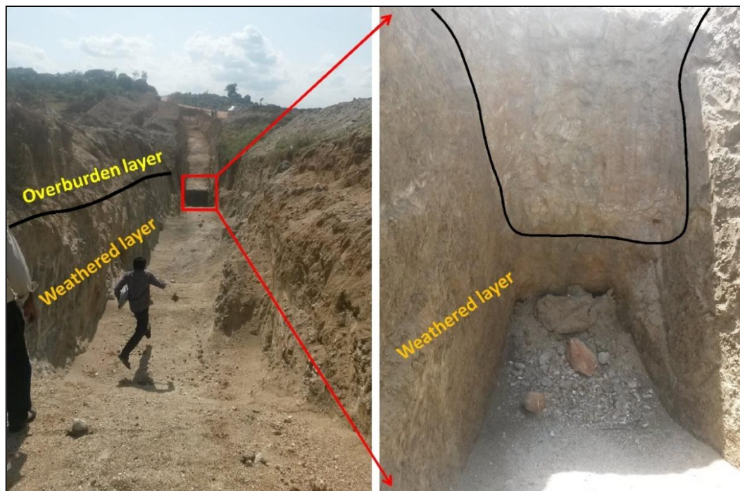
Fig. 2.2 Photograph showing different soil layers clearly and the zoomed area showing the weathered layer deeper in the middle of the trench.
