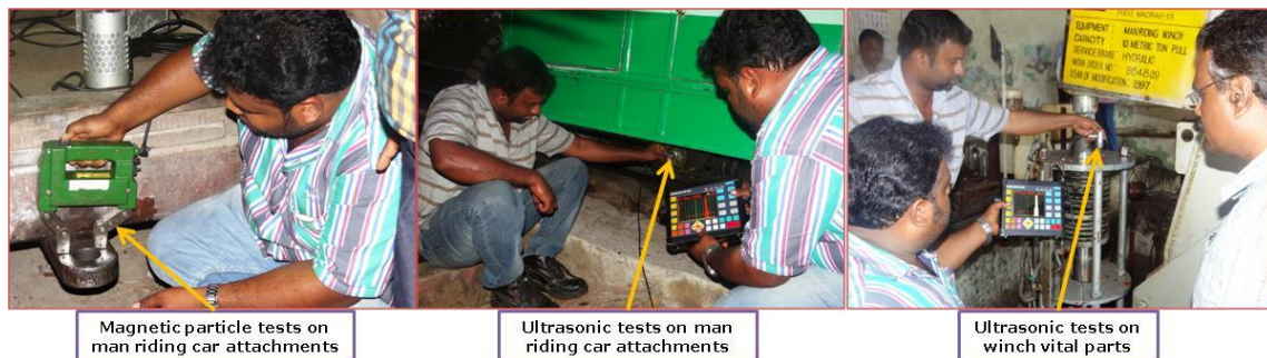
Fig. 8.13 NDT on winch vital parts and man riding car attachments, M/s ADST
