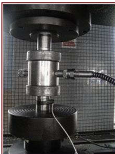
Fig. 68: Triaxial Compression test for Shear strength and Angle of friction
