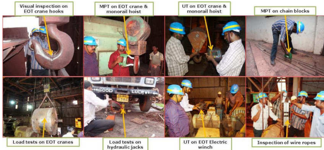
Fig. 63: NDT, proof load tests and wire rope defectograph studies on EOT cranes, monorail hoists, chain blocks, electric winch & hydraulic jacks, M/s NMDC, OCSL Plant.
