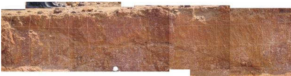
Fig. 36: Gentle south dipping fracture filled with clay observed in the Eastern wall of eastern trench
