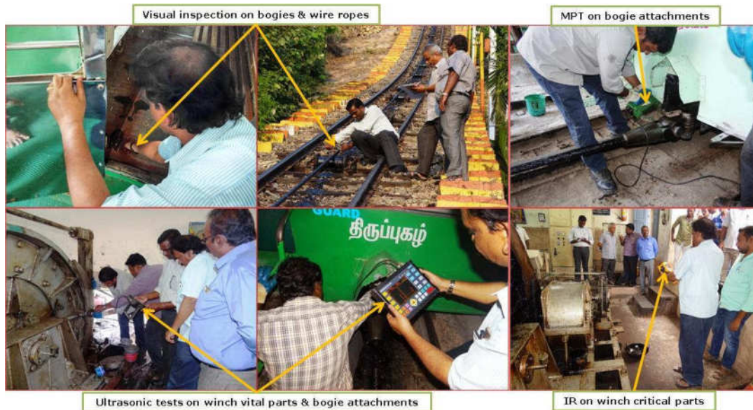
Fig. 55: NDT on winch vital parts, bogie attachments & wire ropes, M/s ADST.
