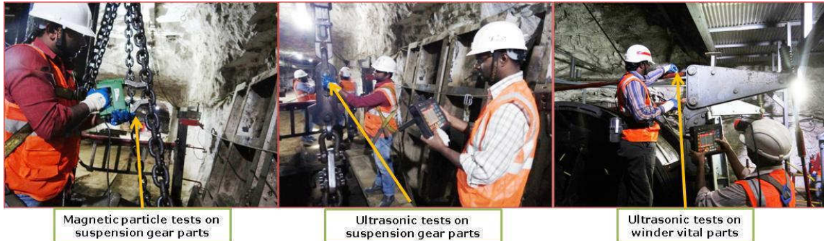
Fig. 58: NDT on winder vital components & suspension gear parts, Zawar Group of Mines, M/s HZL.
