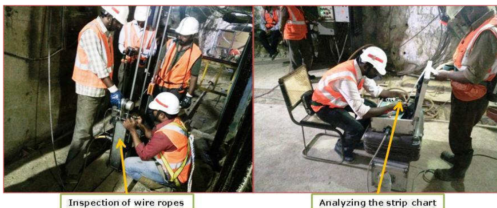
Fig. 59: Inspection of wire ropes, Zawar group of mines, M/s HZL.
