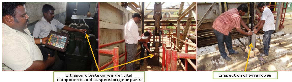
Fig. 64: NDT on winder vital components, suspension gear parts and wire ropes, M/s HCL.
