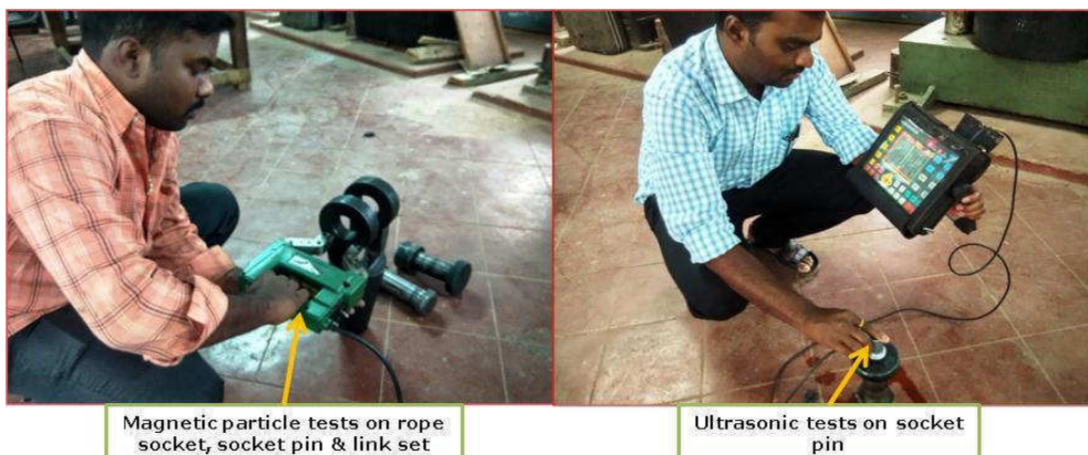
Fig. 54: NDT on rope socket, socket pin & link set at NIRM lab, M/s ADST.
