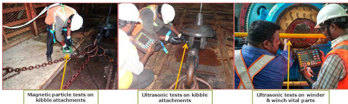
Fig. 60: NDT on winder/winch vital components & kibble attachments, M/s SSM.
