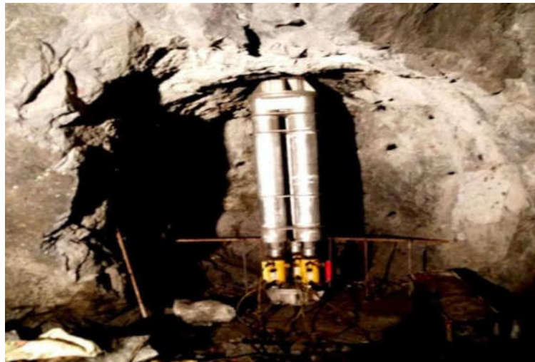
Fig. 11: Complete setup of plate load equipment PCLIS Package-6
