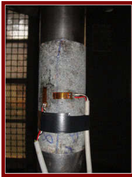
Fig. 67: Uniaxial Compression test for strength and elastic constants
