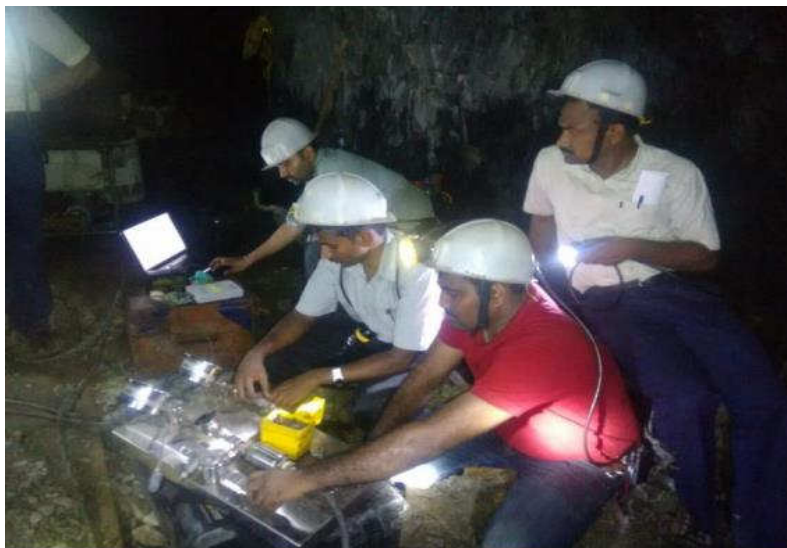
Fig. 9: Execution of Hydrofracture test at Hutti Gold Mine (26 th level)
