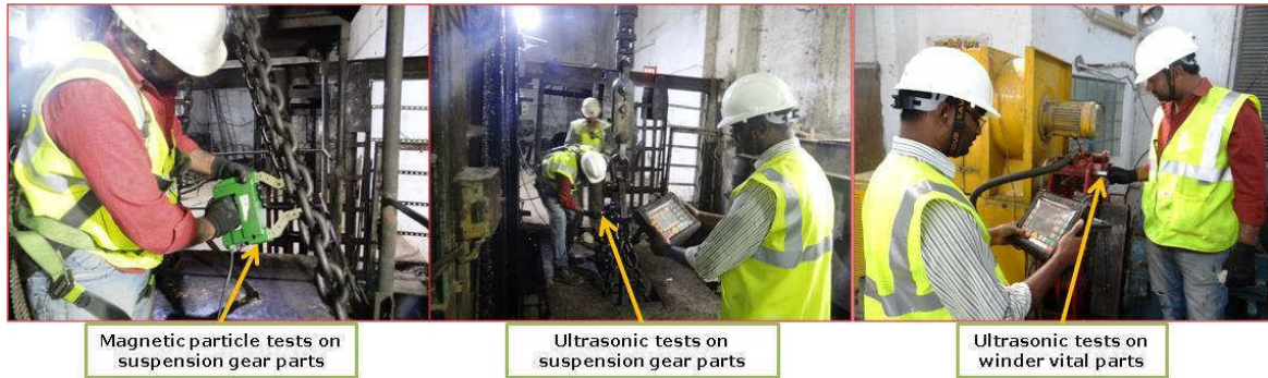
Fig. 56: NDT on winder vital components & suspension gear parts, Rajpura Dariba Mines, M/s HZL.
