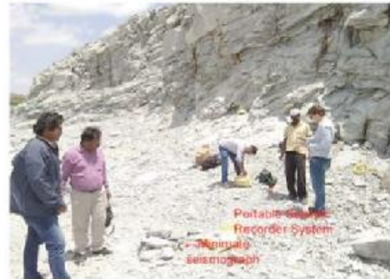
Deployment of Portable Seismic Recorder Systems and Blasting seismograph for a calibration study at a stone quarry.
