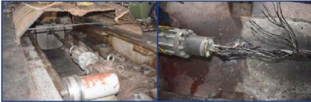
Break Load on suspension device of production and service shaft, M/s SSM
