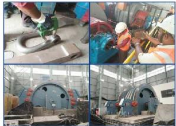
NDT on winder/winch vital components & kibble attachments
