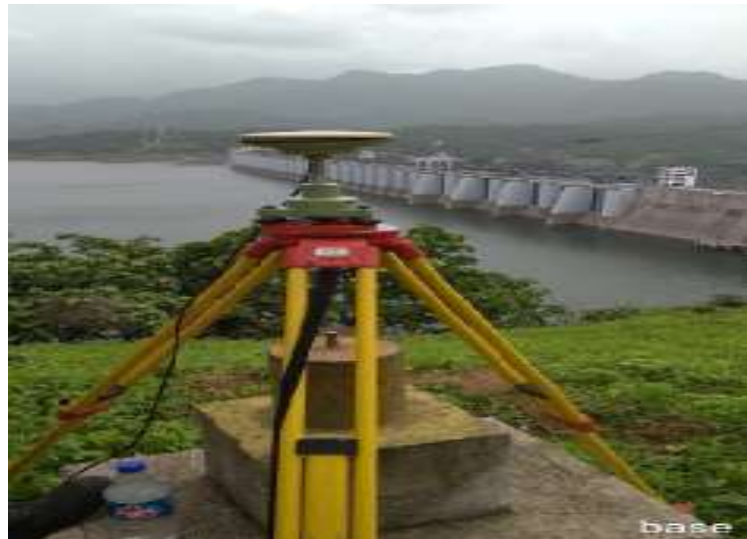
Control Point Survey at DGPS/1
