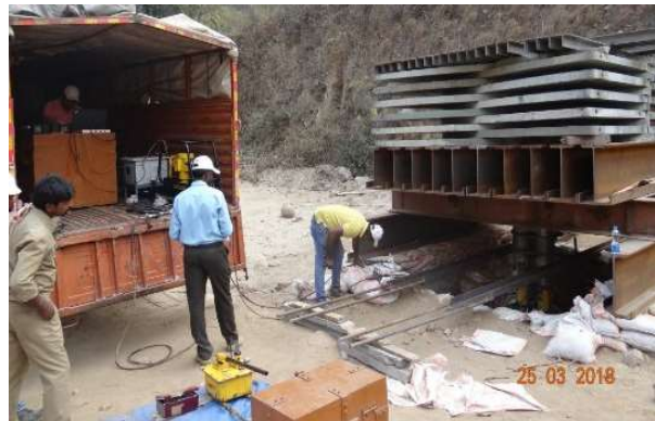
Setup for the Determination of Safe Bearing Capacity
