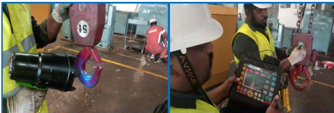
Magnetic particle & Ultrasonic testing on chain pulley hook
