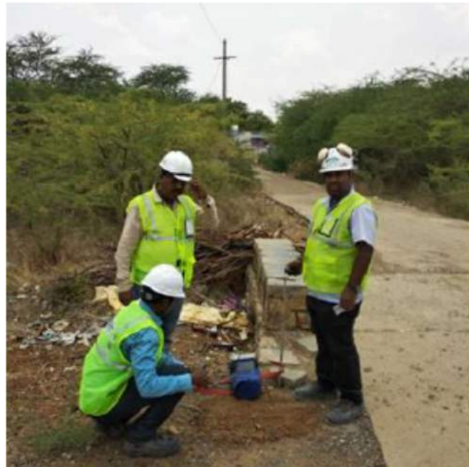
Monitoring ground vibration and air overpressure near western entrance of Valasapalli village
