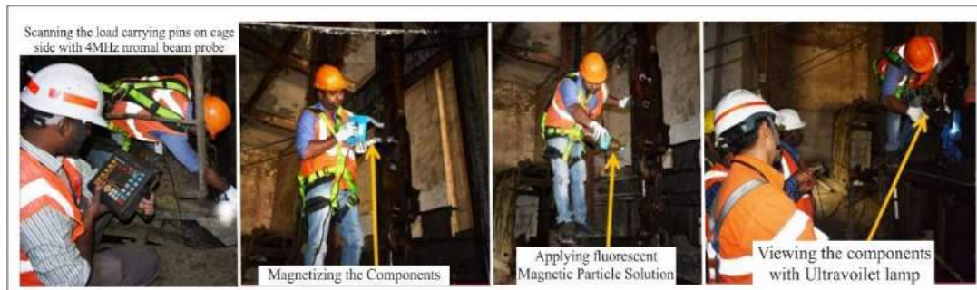
NDT on winder vital components and on suspension gear parts at Rajpura Dariba Mines, M/s HZL.
