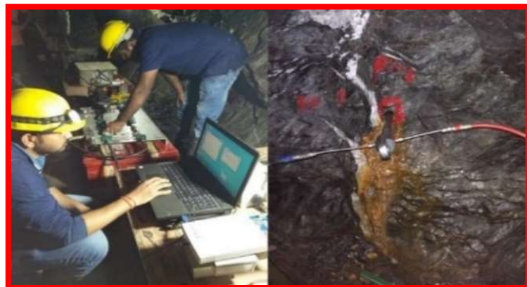
Execution of hydraulic fracturing test at borehole no 1
