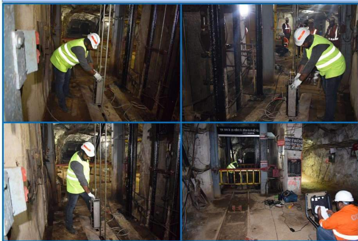
Inspection of wire ropes at Underground Mines of M/s HZL.
