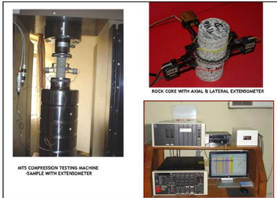
MTS Compression Testing Machine, Extensometer and Data Acquisition System
