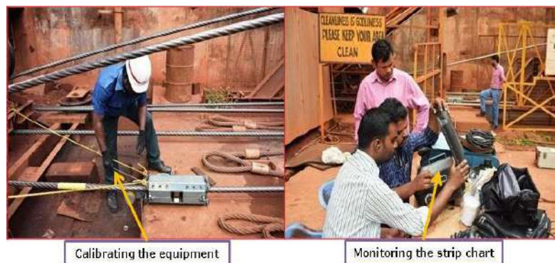
Inspection of Left side rope
