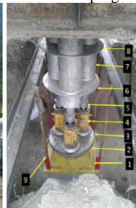
Plate load test setup for determining safe bearing capacity
