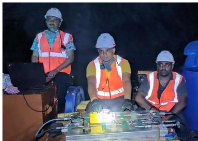
Hydraulic fracturing test at Sindesar Khurd Underground Lead-Zinc mine (HZL)
