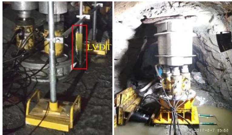
In-situ deformability, Shear and Stress measurements at Arun – 3 HEP, Nepal
