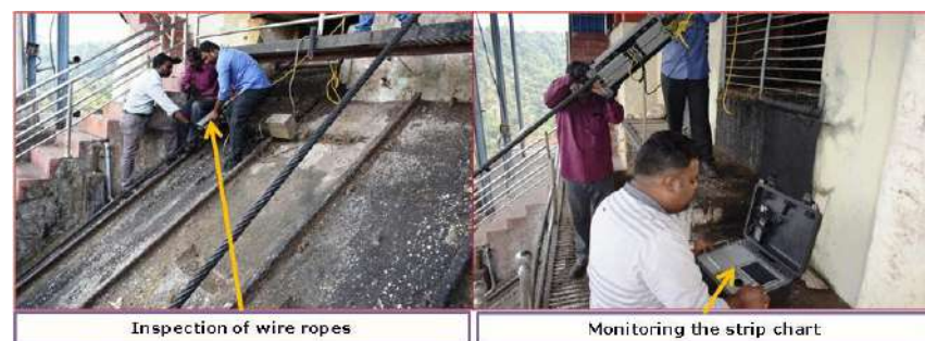
Inspection of wire ropes, M/s KPCL, Jog Falls
