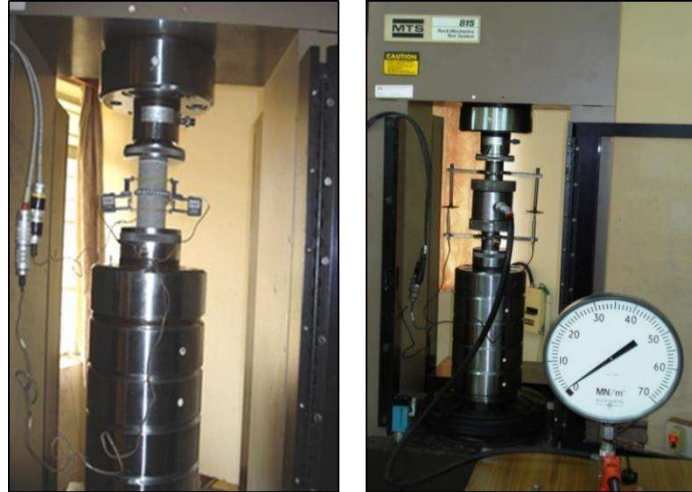
Test setup for uniaxial & triaxial compression
