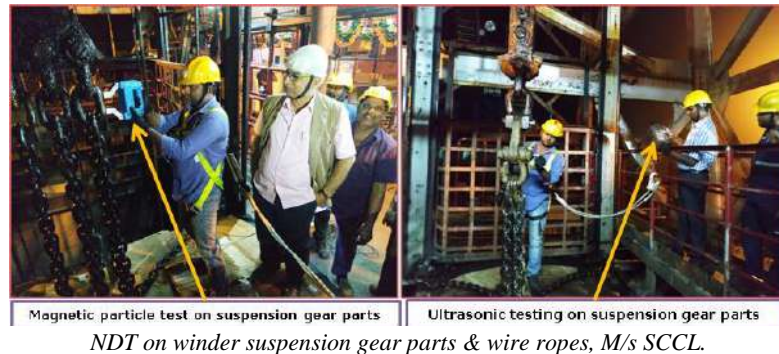
NDT on winder suspension gear parts & wire ropes, M/s SCCL.
