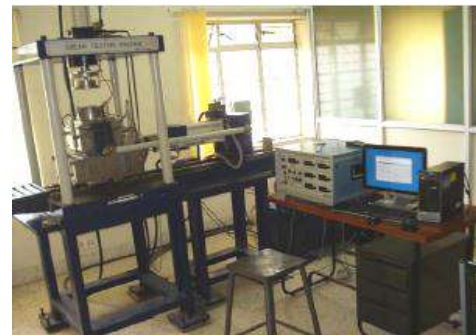
Set up of the direct shear testing equipment with automatic data acquisition system
