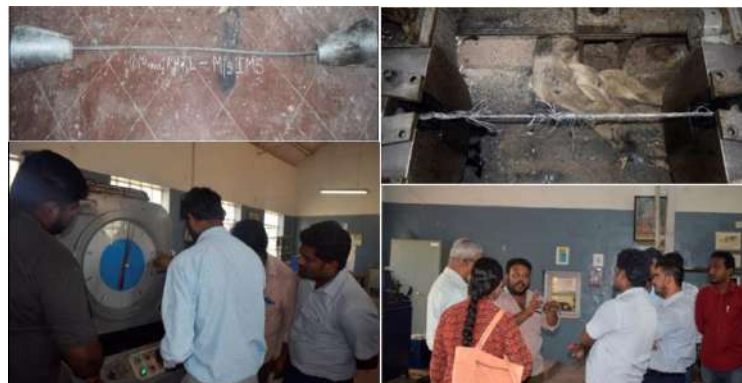
Testing of 14mm, RHL rope and representatives of M/s IMS & Ashok Leyland witnessing the test at NIRM laboratory
