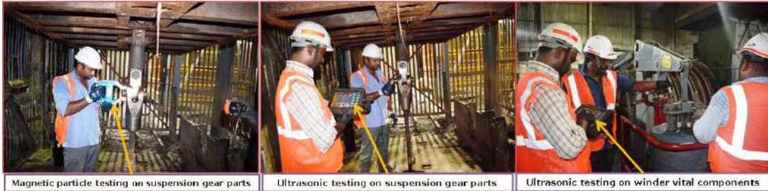
NDT on winder vital components & suspension gear parts, Zawar Group of Mines, M/s HZL.
