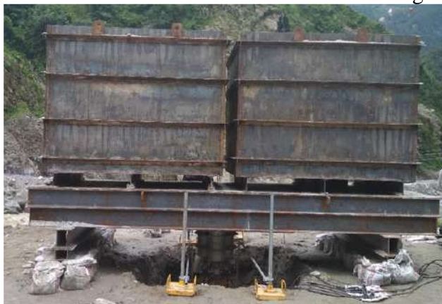
Plate load test setup for determining safe bearing capacity
