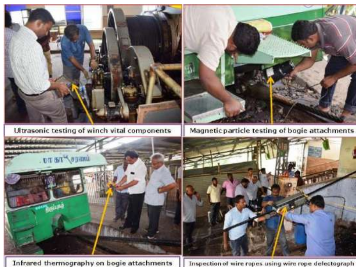
Testing of winch vital parts and bogie attachments
