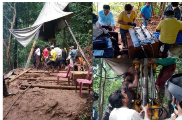
Hydraulic fracture test in progress at DH-7 location
