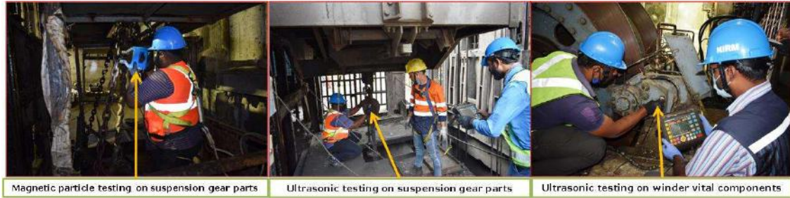
NDT on winder vital components & suspension gear parts, Rajpura Dariba Mines, M/s HZL
