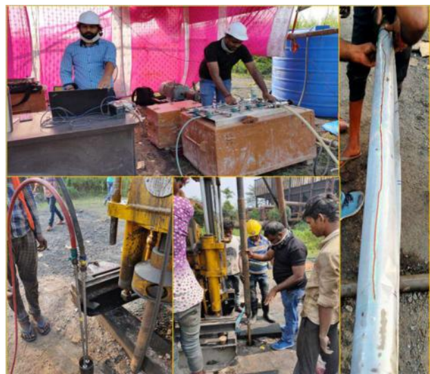
Hydraulic fracture test at BH-02, Nico plant
