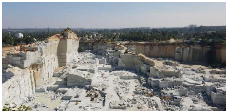
A view of the quarry working by benches
