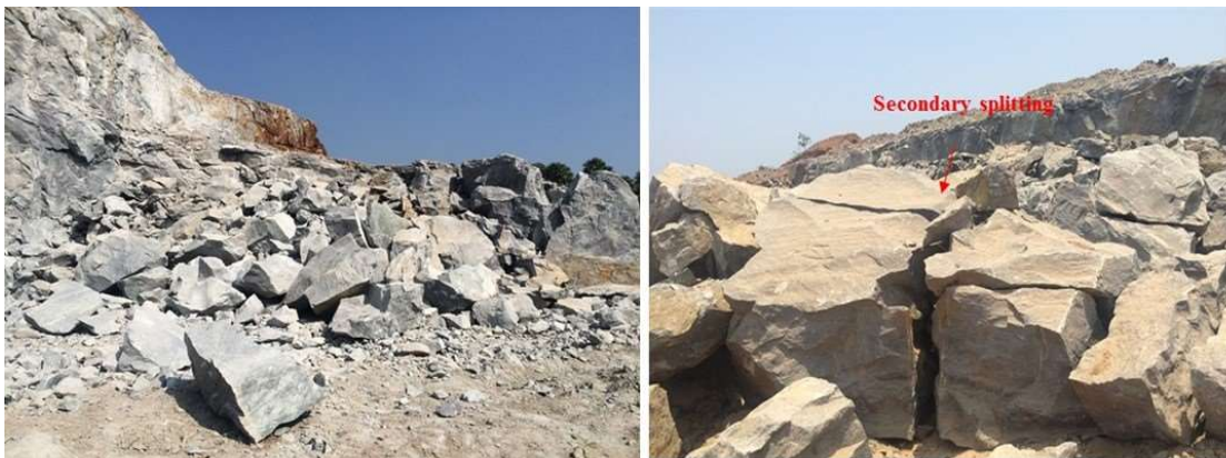
Result of primary blast (left), secondary splitting (right)
