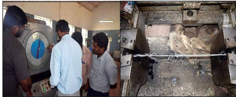
Testing of 14mm, RHL rope witnessed by representatives of M/s IMS & Ashok Leyland at NIRM laboratory
