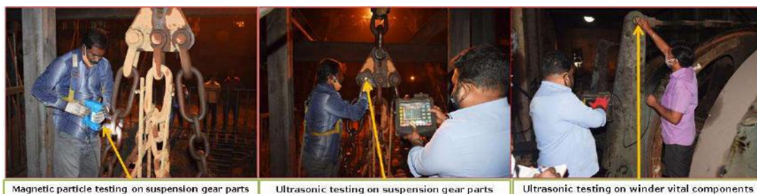
Testing of winder vital components and suspension gear parts
