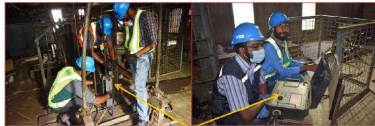
Inspection of wire ropes, Rajpura Dariba mines
