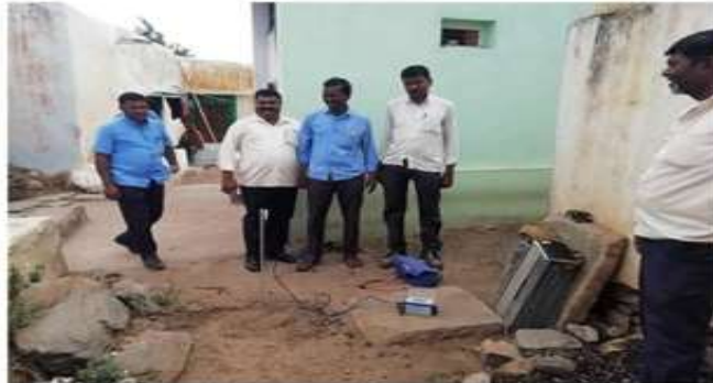
Ground vibration monitoring near Buddini village
