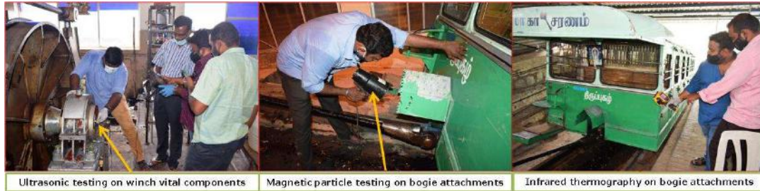
Testing of winch vital parts and bogie attachments
