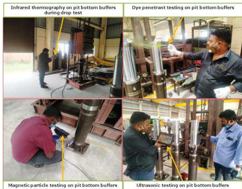
Testing of pit bottom buffers
