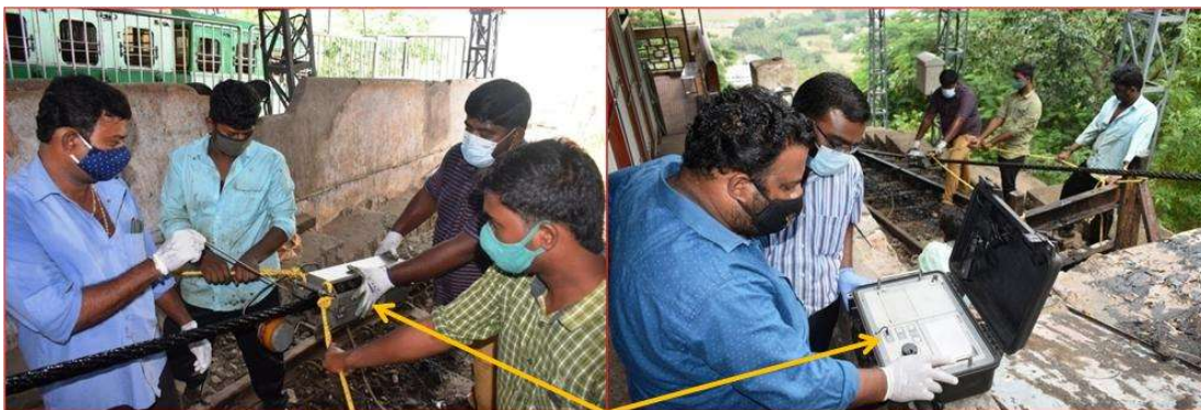
Inspection of wire ropes using wire rope defectograph
