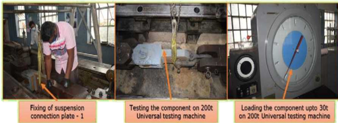
Testing of suspension connecting plate
