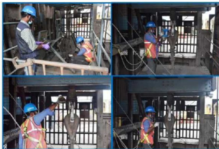
UT and MPT on winder and suspension gear parts.
