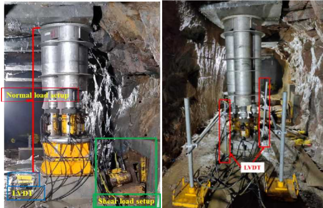
Complete set up of the direct shear test and plate loading test equipment
