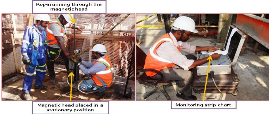
Fig. 8.2 Testing of kibble ropes, rock winder ropes & man winder rope, M/s SSM
