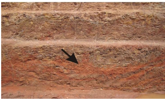
Fig. 1.21 Red bole observed at the bottom of the trench
