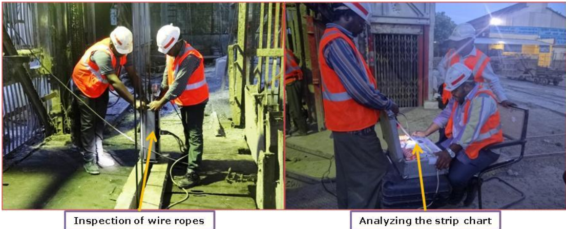
Fig. 8.9 Inspection of wire ropes, Zawar group of mines, M/s HZL
