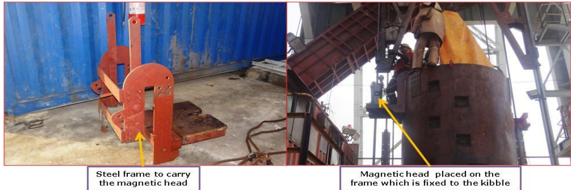
Fig. 8.3 Testing of stage winder ropes, M/s SSM
