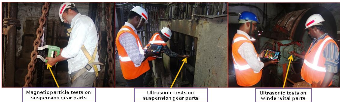
Fig. 8.8 NDT on winder vital components & suspension gear parts, Zawar Group of Mines, M/s HZL
