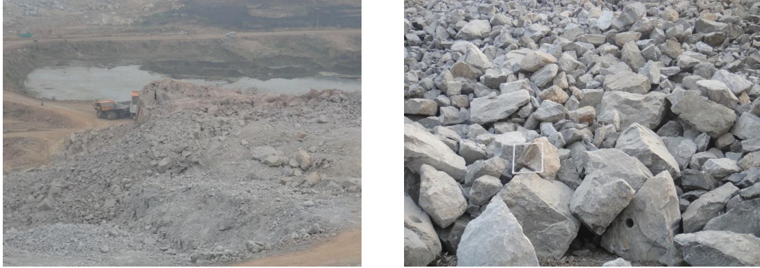
Fig. 6.9 Capturing images for fragmentation analysis
