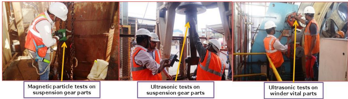
Fig. 8.1 NDT on winder vital components & suspension gear parts, M/s SSM
