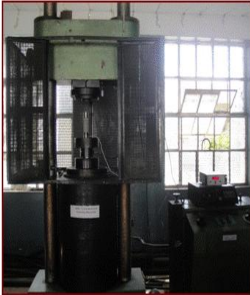
Fig. 8.21 Compression testing set up and Data Acquisition System
