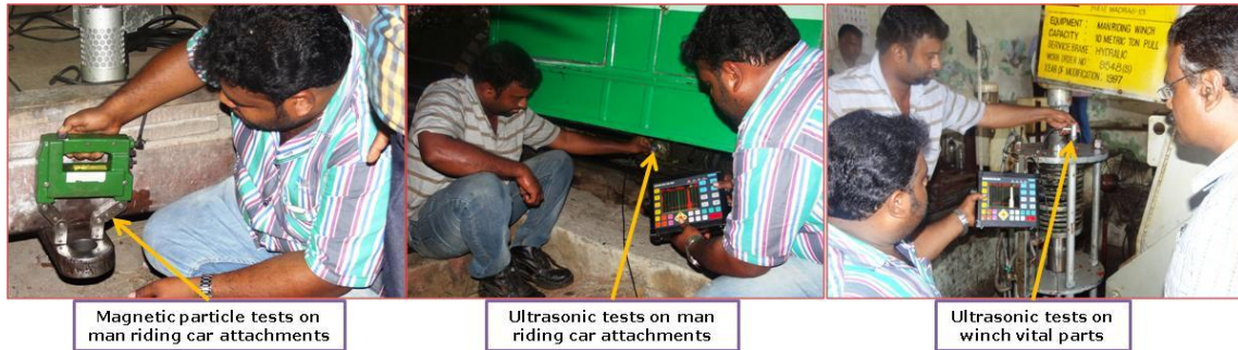
Fig. 8.12 Inspection of wire ropes, Rajpura Dariba mines, M/s HZL
