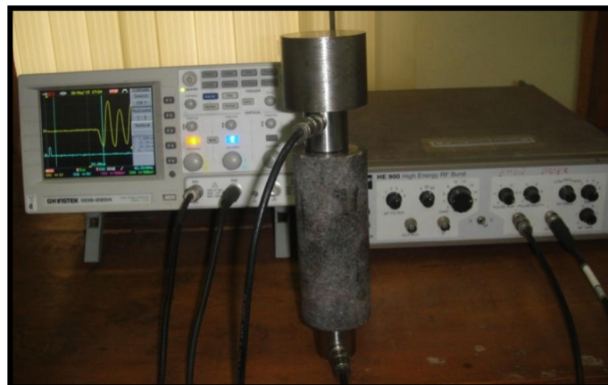
Fig. 8.20 Ultrasonic pulsar, probe and oscilloscope
