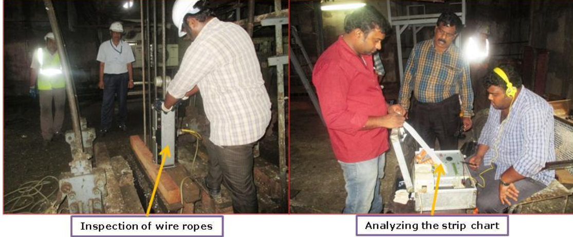
Fig. 8.12 Inspection of wire ropes, Rajpura Dariba mines, M/s HZL
