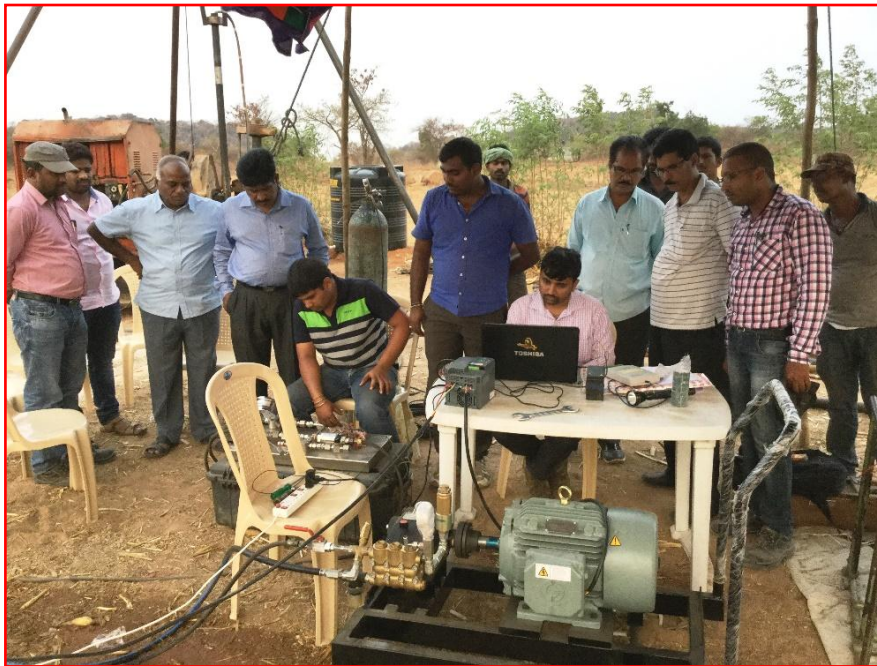
Fig. 3.2 Execution of hydraulic fracture test at Dr B R Ambedkar Pranahitha Chevella Sujala Sravanti Scheme, package – 12
