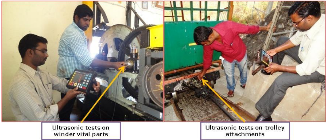
Fig. 8.17 NDT on winder vital components &amp; trolley attachments, M/s KPCL
