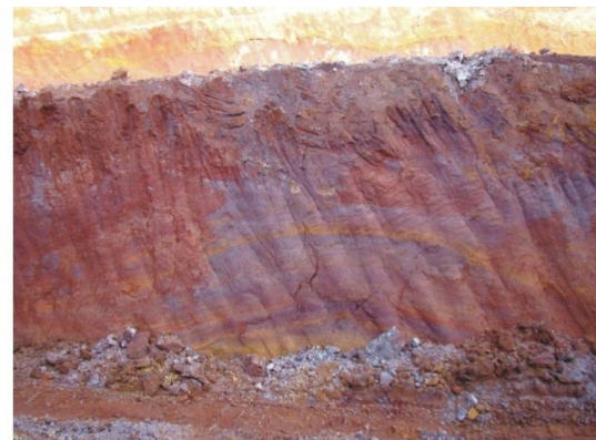
Fig. 1.18 Anticlinal structure observed in the trench face formation
