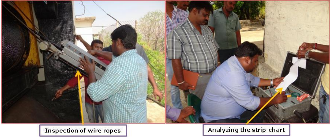
Fig. 8.18 Inspection of wire ropes, M/s KPCL
