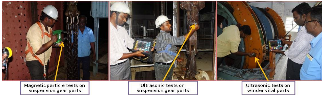
Fig. 8.15 NDT on winder vital components, suspension gear parts, M/s HGML
