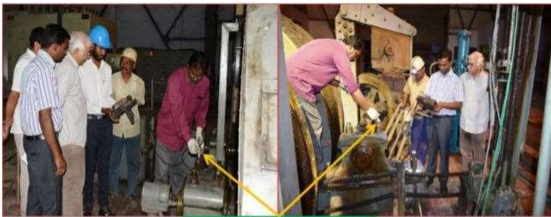
Scanning the pedestal bearing bolts with 2MHz normal beam probe
