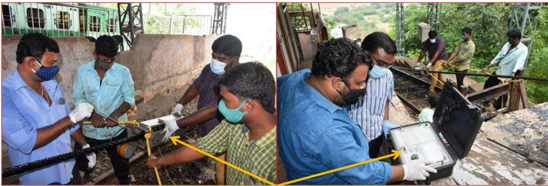
Inspection of wire ropes using wire rope defectograph
