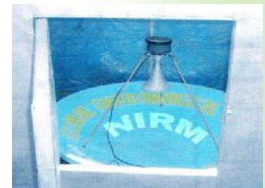
SODAR antenna at a project site
