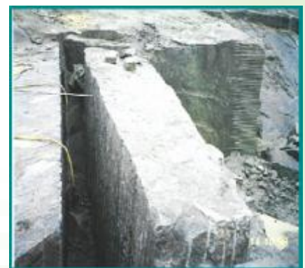
Demonstrating block-splitting of granite
