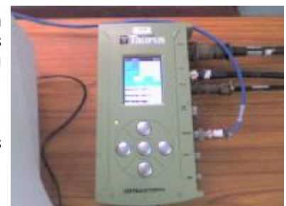
Nanometrics digital seismograph installed for rockburst monitoring
