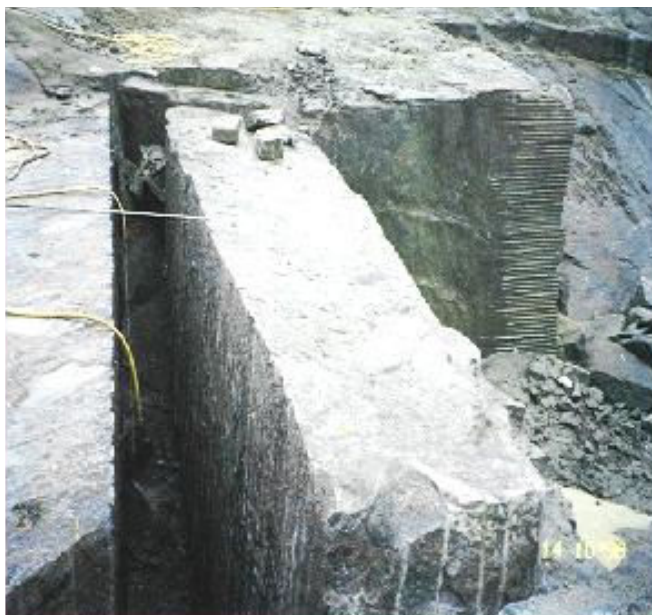
A perfect and smooth face as a result of controlled block splitting
