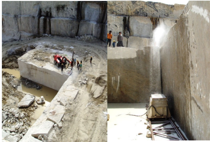
Mechanised drilling of 32 mm dia drill holes and modern wire saw cutting
