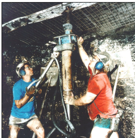
Fig. 3. Mechanized roof bolting system in practice at Tandsi mine, WCL
