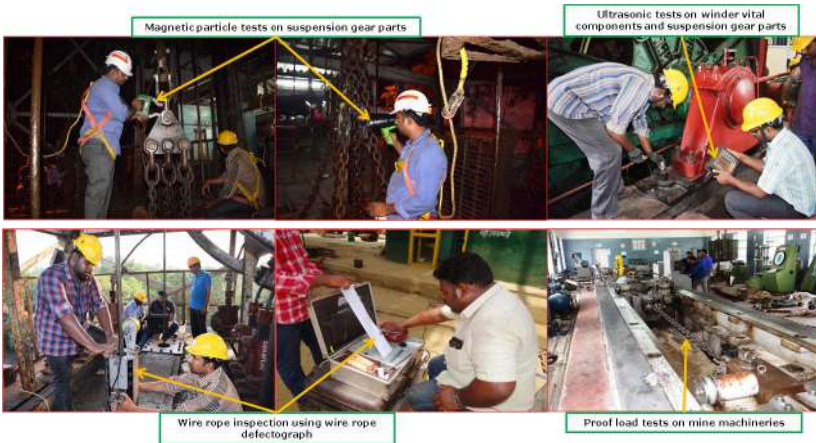
Conducting non-destructive tests on mine machineries.
