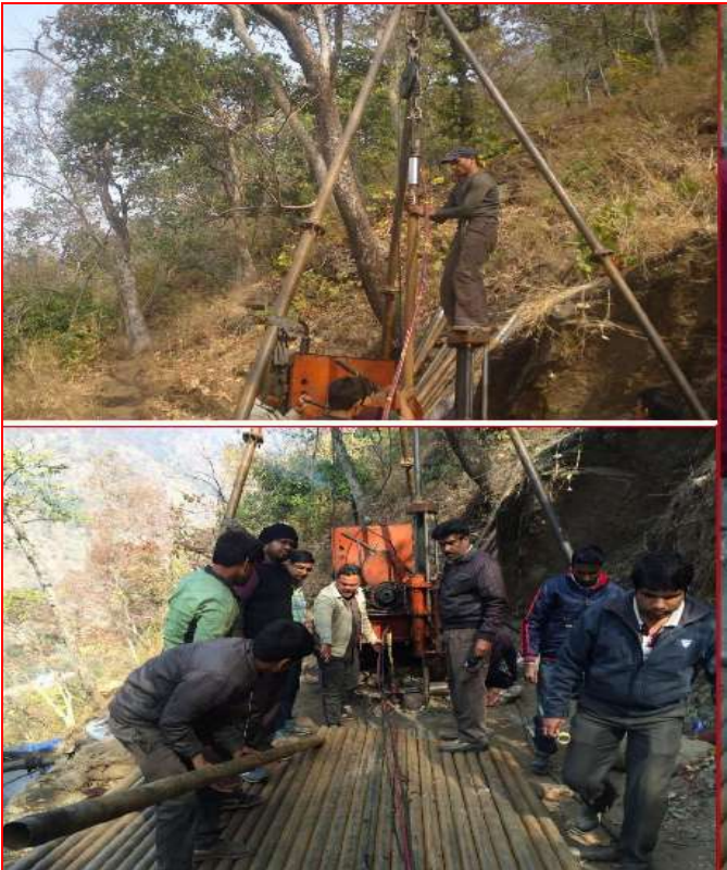
In-situ stress measurement in progress at a coal mining site
