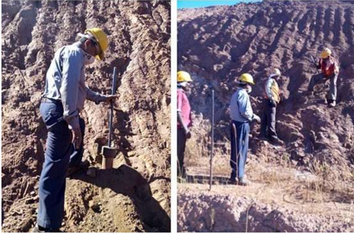
Sample collection for slope stability analysis at an opencast mine site
