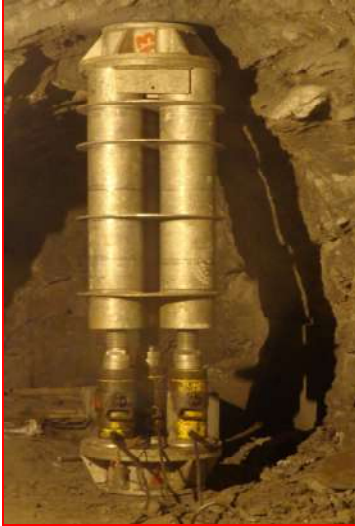
Plate load equipment setup to determine modulus of Deformability
