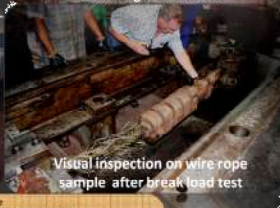
Flowered wire rope ends for socketing white metal
