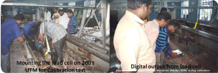
Load cell test setup and cyclic loading of 200 t load cell
