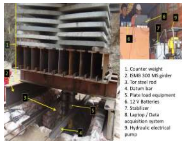
Determination of safe bearing capacity at Punatsangchhu H.E. Project, Bhutan
