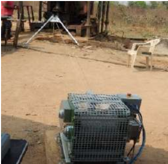
Acoustic Borehole Televiwer tests at the depth of 600m at Singareni Collieries
