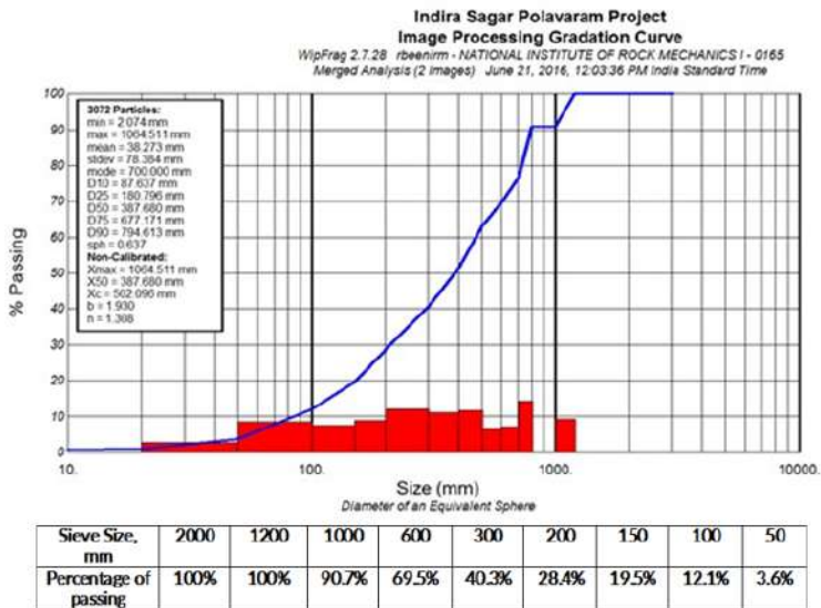
Fragmentation analysis results of a stone quarry
